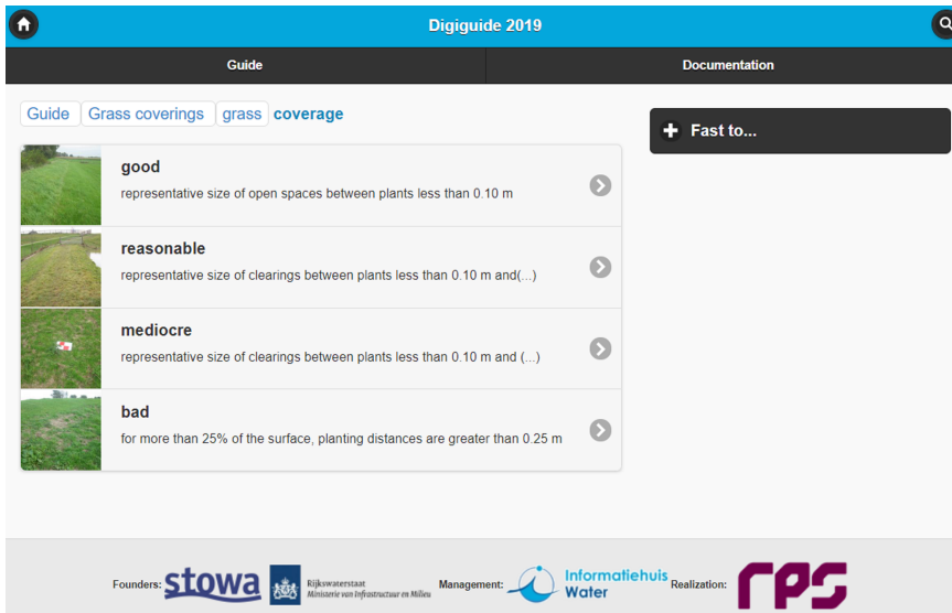
Figure 1.1: Grass cover quality in the Netherlands is assessed based on this table (Digiguide (2019) translated by Google Translate). Digiguide (2019) aids inspectors by providing a database of reference figures to assess the visually observed cover quality based on them.
