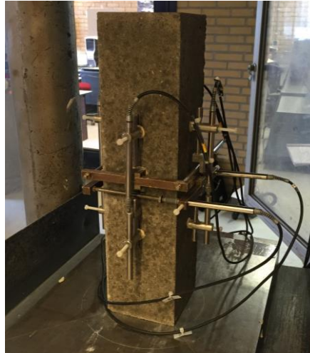
113 Figure 1. Testing set-up for elastic modulus measurement on AAC.
