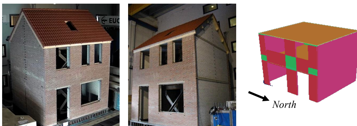
Figure 6: Case study building: North-West (left) and South-West (centre) view (adapted from [13]) and TREMURI model (right)
