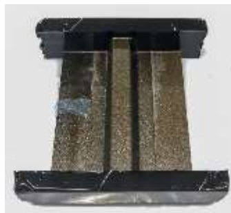
Figure 2. Single-stringer specimens before the test.
