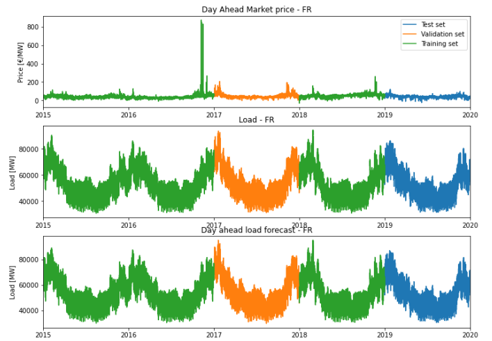
Fig. 2. French historic price, load and load-forecast with train, validation and test splits indicated for model training.
