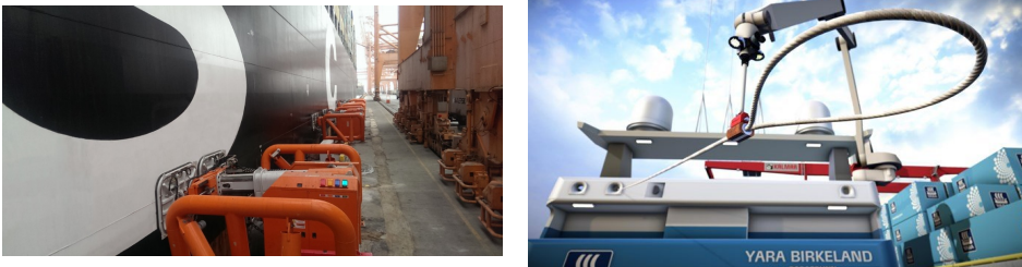
Figure 4.1: Examples of automated mooring systems Left Cavotec's Moormaster [14] and right Macgregor's concept for the Yara Birkeland [47]
