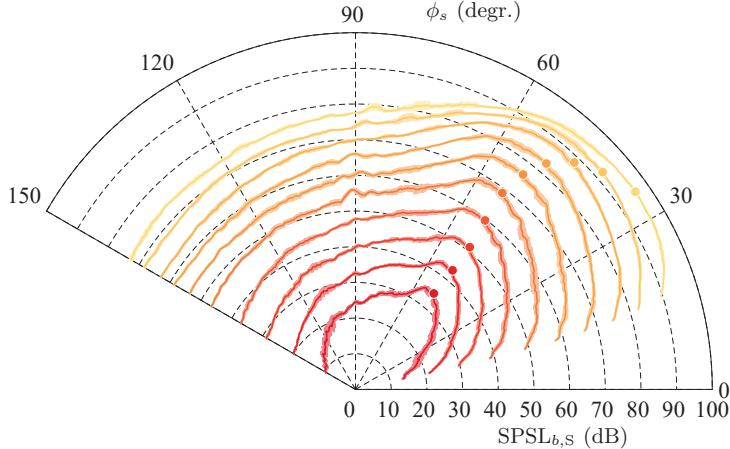
FIGURE 14.  $\text{SPSL}_{b,S}(x, r; \text{St}_b)$  polar patterns at  $\rho_s^* = 60D_j$  for 10 Strouhal numbers, corresponding to bin  $b = 1 : 3 : 28$ . The solid thick lines identifies the average polar pattern; envelopes represent the spread from the root-mean-square of data points while subsequent polar patterns are offset by  $-5\text{ dB}$  (from yellow-to-red).
