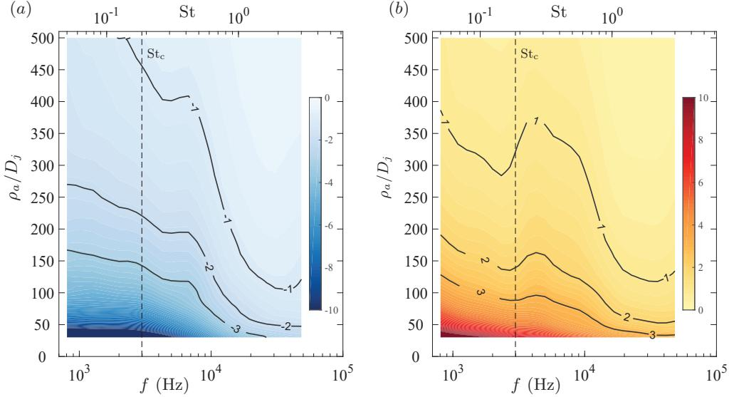
FIGURE 17. (a) Peak negative and (b) positive errors  $\epsilon$  in dB (the asymptotic error taken as the result of the nozzle centred projection, minus the correct polar-pattern based projection), as a function of the nozzle-centered arc radius  $\rho_a$  and for all the frequencies.
