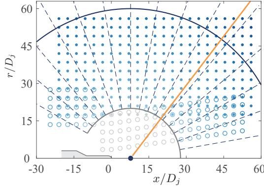
FIGURE 12. Illustration of all measurement points (blue-coloured) used to project SPSL<sub>12</sub>( $x, r; \text{St}_{12}$ ) to an arc at  $\rho_s^* = 60D_j$  and centred at its unique source location. Points with a polar distance  $\rho_s < 20D_j$  (grey-coloured) are omitted in this procedure.
