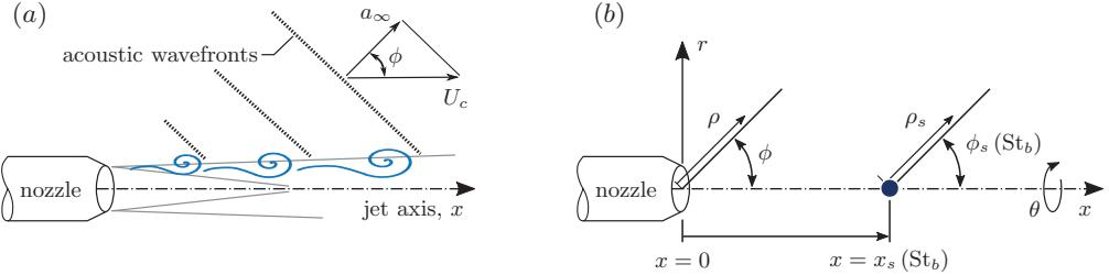
FIGURE 1. (a) Simplified schematic of radiating Mach waves from a jet with supersonic convective Mach number. (b) Coordinate systems pinned to the nozzle exit plane (polar angle  $\phi$  and distance  $\rho$ ) and the frequency-dependent source location (polar angle  $\phi_s$  and distance  $\rho_s$ ).
