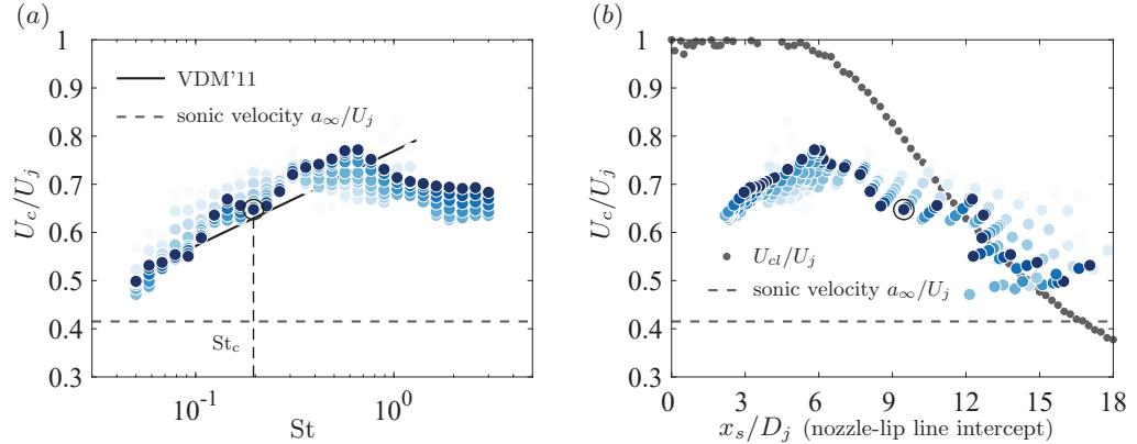
FIGURE 11. (a) Convection velocity versus  $St$ , compared to the trend of Veltin, Day & McLaughlin (2011). (b) Convection velocity versus axial source location, plotted from the data in Figure 10(a) and Figure 11(a). Superposed on this is the centreline velocity profile inferred from Pitot-static pressure and total temperature measurements, described in Appendix A.
