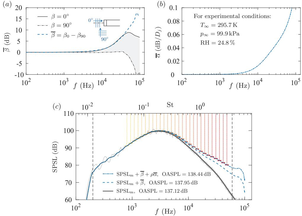
FIGURE 6. (a) Method for calculating free-field microphone correction. (b) Sample atmospheric absorption correction curve  $\overline{\alpha}$ . (c) Sound pressure spectrum level at  $(x, r)/D_j = (35, 39)$ . The OASPL values provided correspond to spectral integrations between the vertical dashed lines at  $f = 200$  Hz and  $f = 60$  kHz. Twenty-eight logarithmically-spaced lines in the range  $0.05 \leq St \leq 3$  identify the centre Strouhal numbers for the analysis described in § 3.1.
