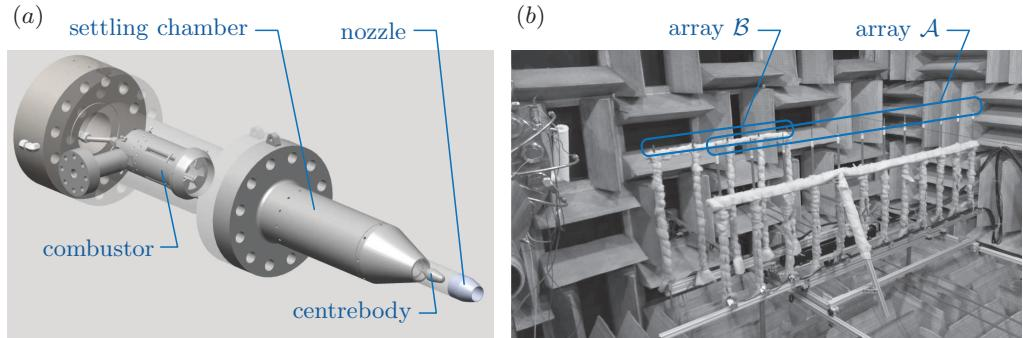
FIGURE 2. (a) Nozzle rig in the Anechoic Jet Laboratory (AJL) of the NCPA. (b) Microphone traversing system made up of a primary stage with twelve microphones (array  $\mathcal{A}$ ) and a secondary stage with five microphones (array  $\mathcal{B}$ ), both oriented perpendicular to  $x$ . Array  $\mathcal{A}$  is movable in the  $x$ -direction; array  $\mathcal{B}$  is slaved to array  $\mathcal{A}$  with an additional translation stage in the radial direction.
