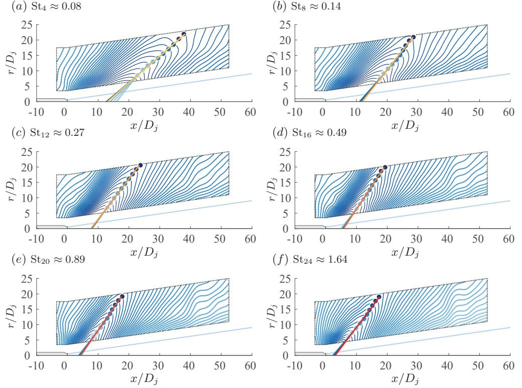
FIGURE 9. (a-b) Spatial maps of  $\text{SPSL}_b(x, r; \text{St}_b)$  for the six bin numbers indicated. Linear fit lines of the ridges identified in the  $\text{SPSL}$  contours are superposed and extrapolated towards the jet axis.
