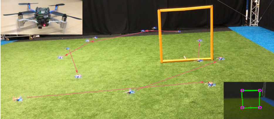
Figure 3.18: Experimental results of coordinated leader-follower flight through a window. Two drones connected with a line are captured at a specific time, where the arrow points to the leader. Only the leader drone is equipped with a monocular camera shown in the left-up corner, and the follower robot maneuvers based on the estimated relative position. The window detection results and its four points are shown in the right-down corner.
