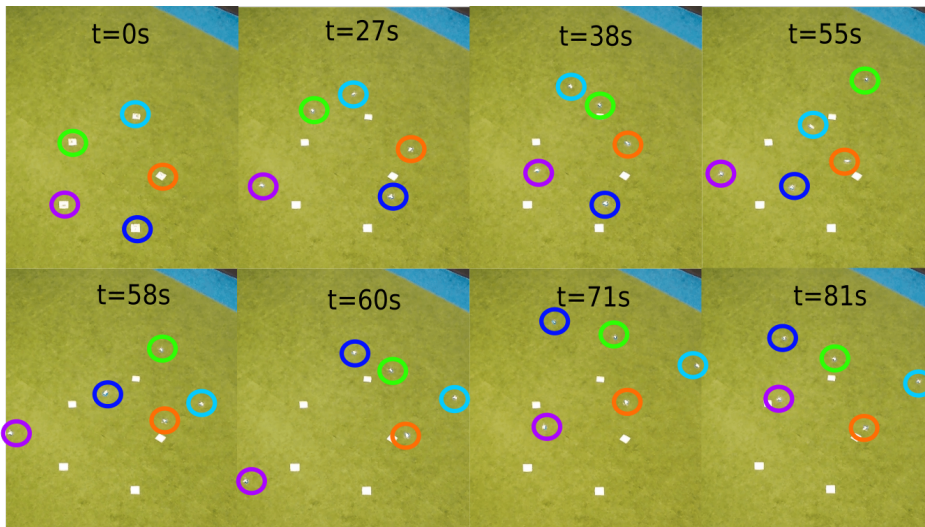
Figure 3.16: Top view of the formation flight of 5 robots. Nine figures show different flight status such as take-off, initialization procedure, distributed control for formation flight, and hovering. Five circles with different colors show the positions of five tiny drones, respectively. Full flight details can be found in the video link https://www.youtube.com/playlist?list=PL_KSX9G0n2P9sgaX3DHnPsnBCJ76fLNJ5
