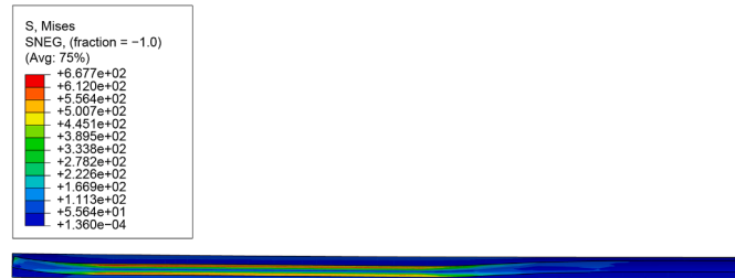
Fig. 8. FEA visualization of EC 3, having a clearance of 0.29 mm. The curved course of the stylet inside the cannula and the corresponding Von Mises stress are shown.
