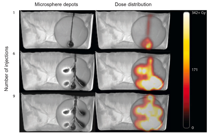
Fig. 11. Microsphere depots and dose distribution in brain tumour phantom visualized by a multi-gradient echo MRI scan (left) and in Q-suite (19.6% Holmium-165 by mass, fictional specific activity 12 MBq/mg) (right). Both images are merged with the T2W-TSE scan for visualization of the instrument and anatomical tumour reference. The administration device has been inserted into the tumour phantom at different locations following the protocol described in Section 2.2.3. After nine injections the total mean dose is 66 Gy, of which 40% of the tumour volume received a dose of at least 60 Gy.
