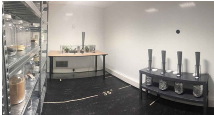
FIG. 3.1 Air Quality Chamber: CLIMPAQ 50L and sniffing table.
