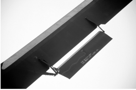
FIGURE 2. FLAP USED IN KAMAN HELICOPTERS.
