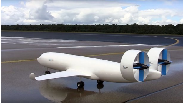
Fig. 1 Subscale test article of aircraft with fuselage-mounted ducted propellers prior to demonstration flight.
