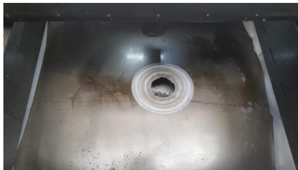
Fig. 9. Damage removed using the MobileBlock.
