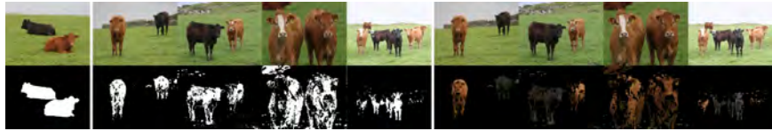
(b) Segmentation with parameters \varepsilon = \tau = 0.00025, K = 100, k_b = 1, k = 1, \hat{\mu} = 500, \sigma = 35 , and the symmetric normalised Laplacian. Elapsed time for segmentation: 14.0 sec.
