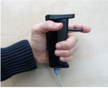
Fig. 7: The push-button interface used to command robot endpoint stiffness from [8], [26]. Because the original interface could only scale the size of the stiffness ellipsoid in all directions simultaneously, we upgraded it with a multi-modal system, where the user can switch the modes for scaling orientation and major and minor axes. The upgraded push-button interface is comparable in price and applicability to the novel tablet interface and is therefore used as a benchmark in the multi-subject analysis.
