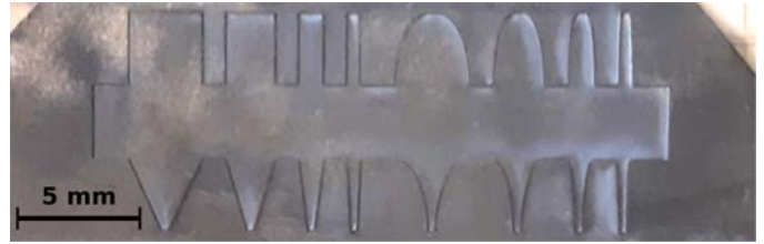
Fig. 4. IPMC sheet after laser cutting. The separated monolithic IPMC sample consists of clamping region (middle portion) and actuation units (top and bottom rows). The clamped sample is shown in Fig. 10.
