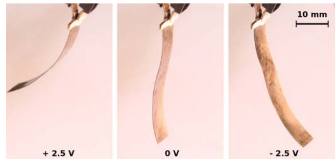
Fig. 1. IPMC actuation: the material at rest (center), and with 2.5 V applied at opposite polarities (left and right).
