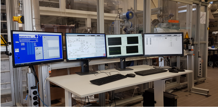
Figure 5.11: The control and monitoring station of the ORCHID. The computer monitors display graphical user interfaces of the ORCHID CODAQ software.
