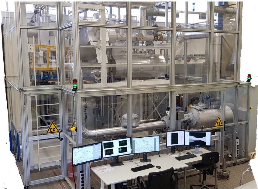
Figure 2.19: The ORCHID located in the Aerospace Propulsion and Power laboratory of the Delft University of Technology. The surrounding structure is a ventilation cabinet containing the BoP and TS together with the measurement systems. Photographed by Henk-Jan Siemer.
