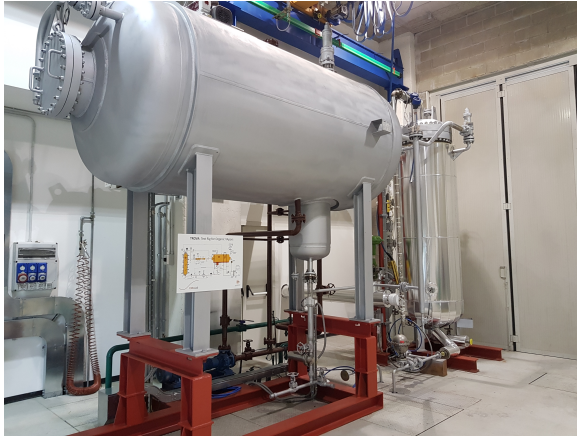
Figure 2.13: The TROVA. The components which can be seen belong to the balance of plant (BoP), e.g., the high pressure vessel, the membrane pump and main valves. The test section (TS) is located in a dedicated room together with the measurement system. Photographed by Adam J. Head in the 4th International Seminar on ORC power Systems.
