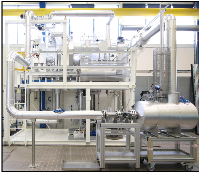
Figure 5.1: The working fluid loop of the ORCHID, before the installation of the ventilation cabinet.
