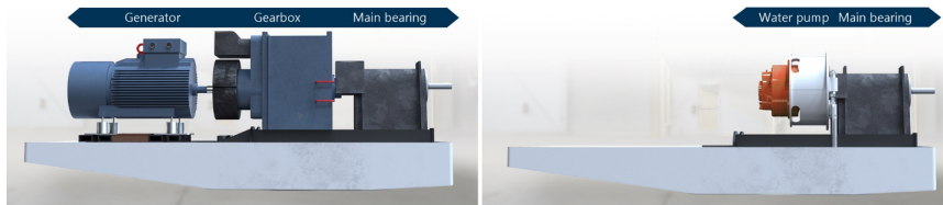
Figure 2.3: Image obtained from [174]. (Left) A conventional lay-out of a gearbox generator wind turbine. (Right) The setup proposed by Delft Offshore Turbine, with its potential weight and space reduction.
