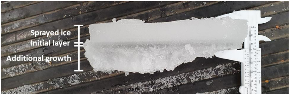
Fig. 4. Ice vertical cross section at the end of a test day (17-6-2021): a sprayed layer on top, a layer of initial ice that was formed before the start of the spraying process in the middle, and a layer of additional ice growth at the bottom, which increases during the day.
