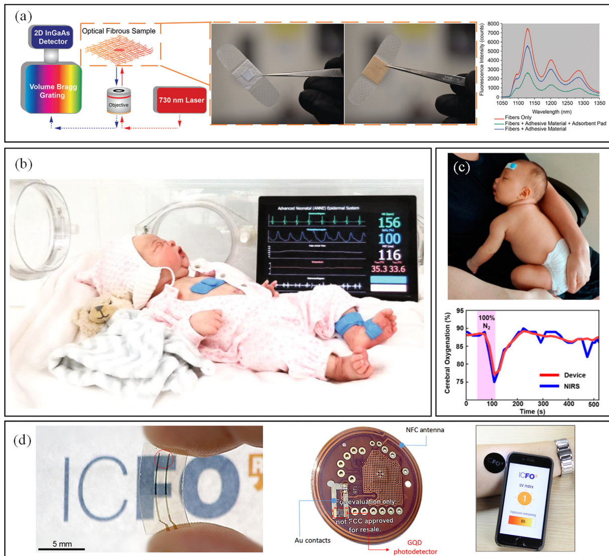
Fig. 2. Portable and wearable electronics for optoelectronic sense: (a) Optical micro fibrous biomaterial with encapsulated nanosensor [97]; (b) Skin-interfaced biosensor for monitoring in neonatal and pediatric intensive-care units [60]; (c) Skin-interfaced biosensor for cerebral hemodynamic monitoring in pediatric care [61]; (d) Flexible and transparent wearables based on graphene sensitized with semiconducting quantum dots [98].
