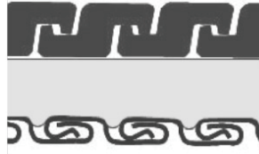
Fig.3 Extrusion of the inner liner into the adjacent interlocked carcass [11]
