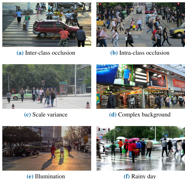
FIGURE 3. Some challenges of pedestrian detection. (a) Inter-class occlusion. (b) Intra-class occlusion. (c) Pedestrian of different scales, small-scale pedestrian in red box and large-scale pedestrian in blue box. (d) Complex background. The dummy in the green box. (e) Illumination. (f) Rainy day and blur.
