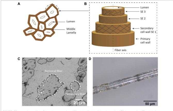
FIGURE 5 | Structure of natural fibers: Schematic representations of (A) technical (fiber bundle from the stem) and (B) elementary fiber, (C) optical microscopy image of technical and elementary fibers in a composite and (D) optical microscopy image of an elementary fiber surface.
