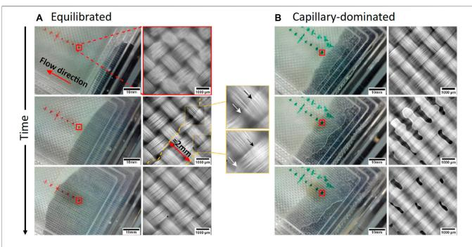
FIGURE 4 | Progressive saturation recorded by synchrotron radiation computed laminography of (A) Equilibrated and (B) Capillary dominated flow regimes (Source: (Castro et al., 2021)).
