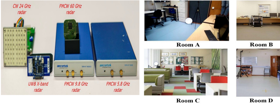
Fig. 1. The left shows the radar systems used by the radar team at the University of Glasgow. They used the rightmost radar, SDR-KIT-580B of Ancortek, to create the open dataset. The right shows four examples of the experiment environments for data collection adapted from [3, 22].
