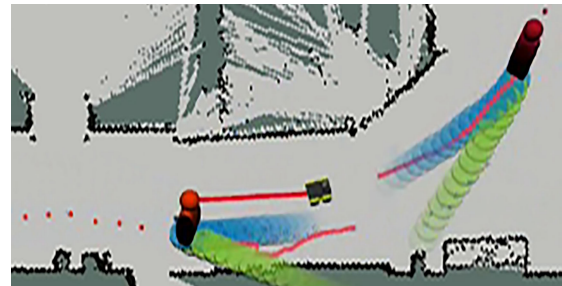
Fig. 7. Map view of the real-world application of SCL on moving robot using on-board perception. The green and blue disks depict the predicted trajectories employing the pre-trained model and the SCL-trained model, respectively. The red dotted lines depict the pedestrians' past trajectories. The pedestrians' and robot's future trajectories are shown as solid red lines.
