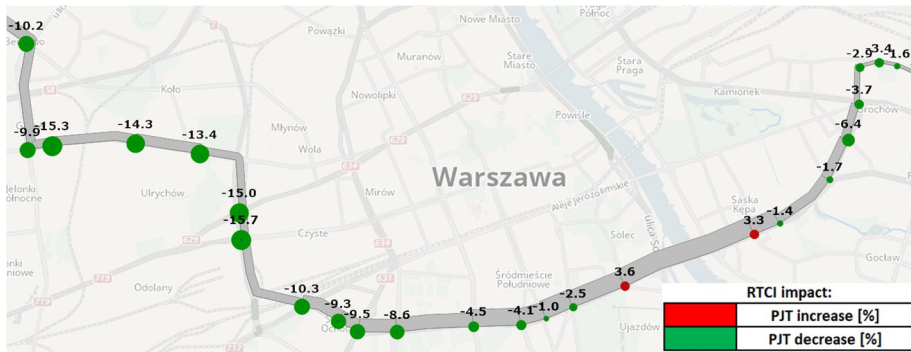
Fig. 9 Relative changes (in [%]) in total travel disutility (i.e. total PJT) in the RTCI scenario, distinguished for passengers boarding at individual bus stops
