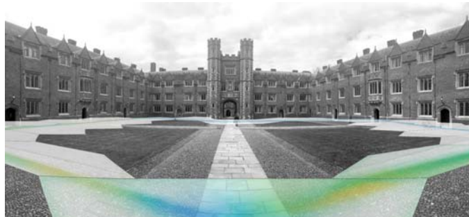
Fig. 1. Illustration of a magnetic field map built using our SLAM approach. Each hexagonal block (with radius of 5 m and height of 4 m) covers a Gaussian process magnetic map volume of \sim 260 \text{ m}^3 in a state dimension of 256. A more detailed map is provided in Fig. 5.
