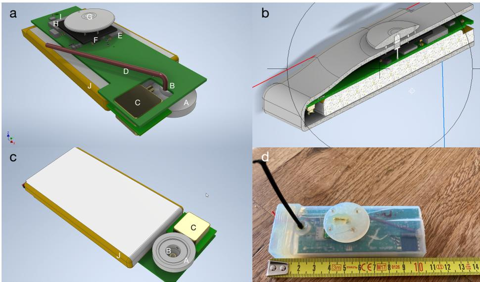
**Figure 2.1:** 3D CAD design of (a) the top of the PCB, (b) the casing, (c) the bottom of the PCB with pressure dome, and (d) a picture of the actual platform. The PCB hosts; a pressure dome (a-A/c-A), a barometric pressure sensor (a-B/c-B), a differential pressure sensor (a-C/c-C), a PEEKsil Red series capillary (a-D), an accelerometer (a-F), an anemometer (a-F) with the heating element (a-G), a microcontroller (a-H), a GPS (a-I), and a lithium battery (a-J/c-J).
