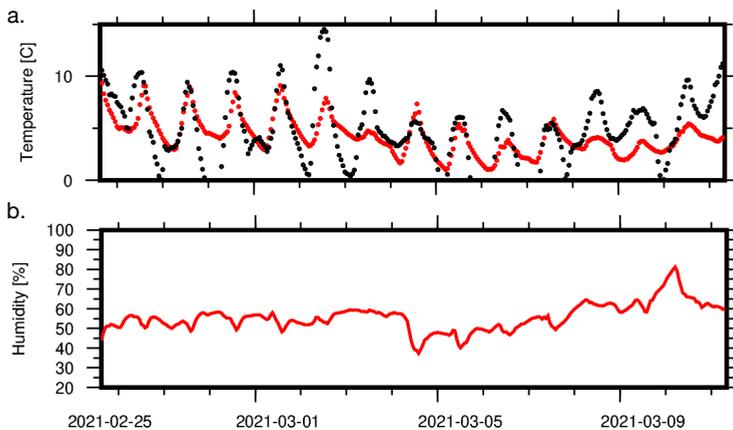
**Figure 2.18:** Temperature and humidity measurements by the Multi-EAR (red) compared to the KNMI reference sensor (black). The measurements are obtained within building K, therefore a correct comparison between the Multi-EAR and KNMI sensors is not possible.
