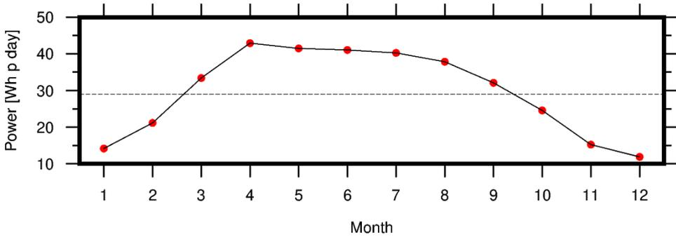
**Figure 2.16:** Performance of the 9Watt, 6Volt, solar panel. The red dots indicate the average daily power provided by the solar panel per day. The dotted line shows the required power per day by the monitoring system. When the provided power is larger than the required power the battery will be charged.
