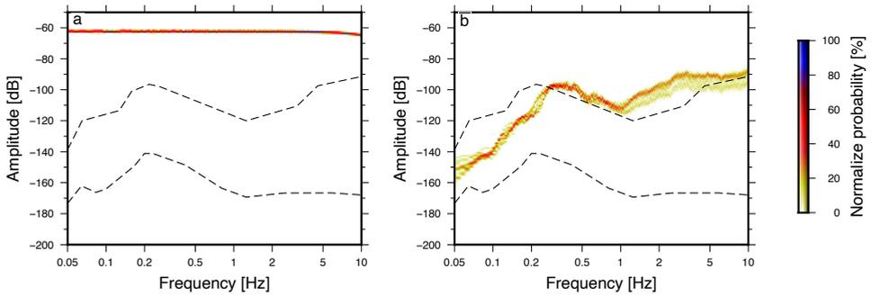
**Figure 2.7:** PPSD's of the LSM IMU accelerometer (a) and the Streckeisen STS-2 connected to a Quanterra Q330 (b) for 24 hours of continuous recording in dB re.  $m^2 s^{-4} Hz^{-1}$ . The dotted lines indicate the seismic high and low ambient noise levels [Peterson, 1993].
