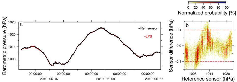
**Figure 2.5:** A comparison between the Barometric MEMS sensor (red) and a KNMI reference barometer (black). Panel (a) shows five days of barometric pressure recordings using both sensors, while panel (b) displays the difference in measured barometric pressure by the MEMS and the reference sensor.
