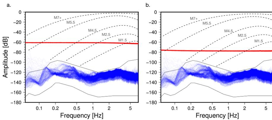
**Figure 2.20:** Power Spectral Density curves, hourly calculated for the LSM (red lines, panel a), the LIS (red lines, panel b), and the reference sensor (blue lines in both panels). The solid gray lines indicate the global high and low ambient seismic noise curves [Peterson, 1993; McNamara and Buland, 2004]. The dotted lines indicate the theoretical amplitude levels of a nearby transient event.
