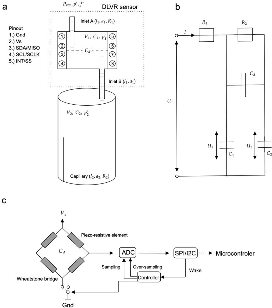
**Figure 2.2:** The KNMI mini-MB design with the DLVR sensor and the parameters as listed in Table 2.1 (a) and the electrical circuit of the mini-MB (b). Panel (c) visualises the DLVR sensor.
