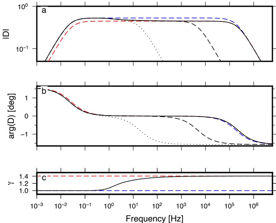
**Figure 2.3:** The theoretical sensor frequency response function for (a) amplitude and (b) phase in the case of isothermal and adiabatic gas behaviour in blue and red, respectively. The solid black line indicates the corrected sensor response by  $\bar{\gamma}$  (c). The dotted and dashed line indicate the high-frequency shifting cut-off due to  $R_{gore}$ .
