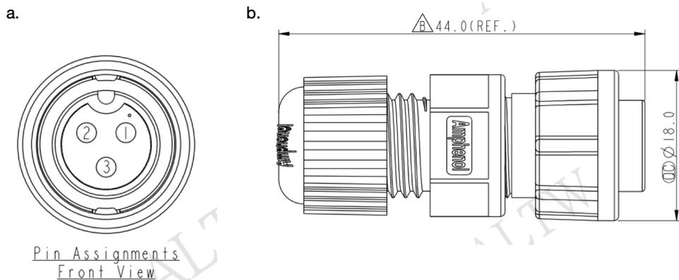
**Figure 2.15:** Amphenol connector. Panel (a) shows the front view of the pin assignment. Pin 1 is the power supply, Pin 2 the ground, while Pin 3 remains available. Panel (b) shows the side view of the connected male and female connector.
