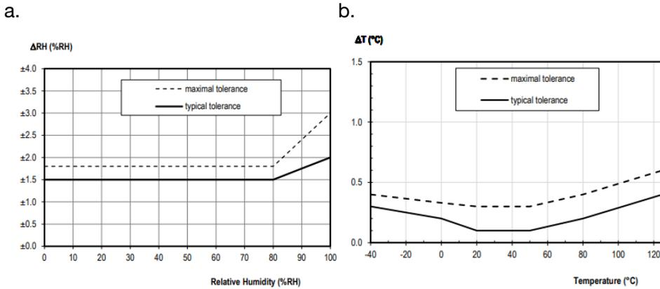
**Figure 2.11:** Sensitivity curves of the SHT3x MEMS sensor. Panel (a) shows the expected tolerance of the humidity sensor over the measurement range. Panel (b) shows the tolerance of the temperature sensor.
