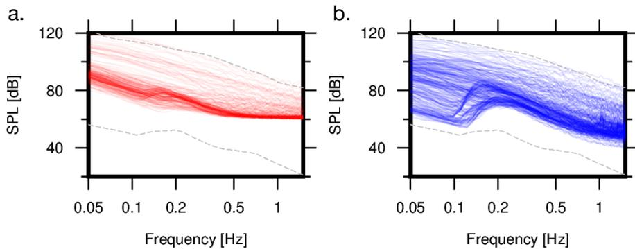
**Figure 2.19:** *Infrasonic wavefield measurement by the KNMI mini-MB (panel a) and a Hyperion IFS-5100 (panel b). The gray dotted lines indicate the global high and low noise curves [Brown et al., 2014]. Note that both sensors resolve the characteristic microbarom peak around 0.2 Hz. At the higher frequencies, the self noise levels of the KNMI mini-MB dominate the measurements.*
