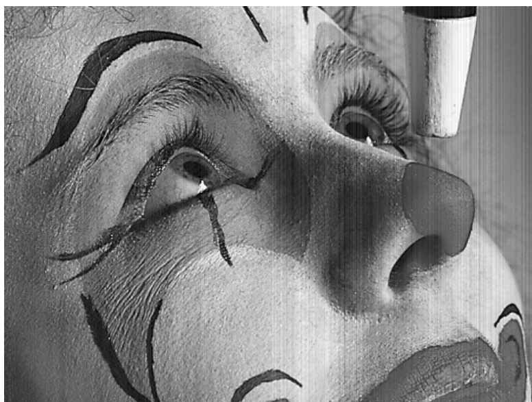
Figure 4-22: Sample image with 3% Gaussian column FPN. DCS is simulated on the left half of the image using the improved switching cell of Figure 4-21
