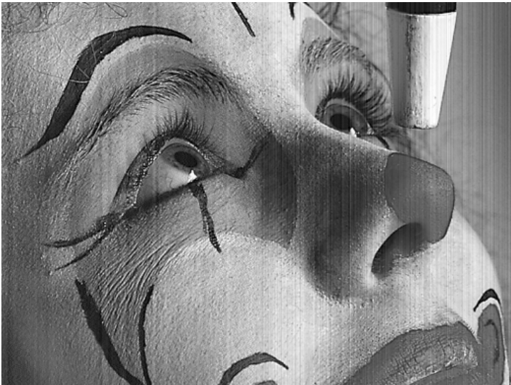
Figure 4-18: Sample image with 3% Gaussian column FPN. DCS is simulated on the left half of the image using a 3x3 unit switching cell
