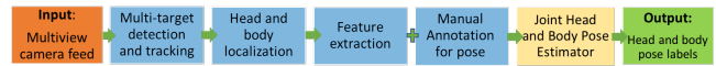
Figure 2: Overall work flow of this study. The focus of this study is highlighted in yellow
