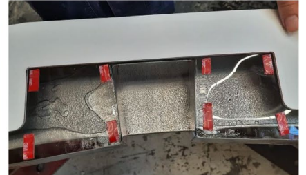
4. Double-side tape spacers are placed at the edges of the brick below.
