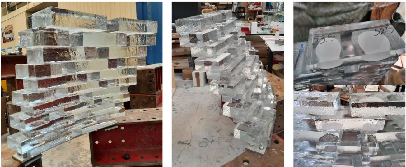
Fig. 18 Prototype constructed at the TU Delft Glasslab, showing the natural tilt of the bricks due to the larger cantilevering width in the initial design (left and center). The application of the DOWSIL
