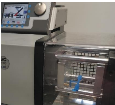
Fig. 3. Injection moulding of dog bones in various mixing ratios.
