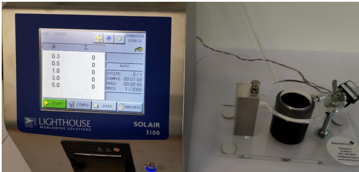
Fig 2. Lighthouse Solair 3100 particle counter connected to a particle chamber.
