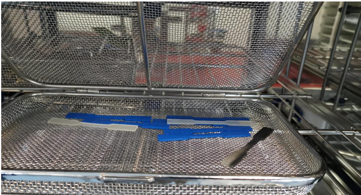
Fig. 1. Dog bones cleaned & disinfected during ten cycles.
