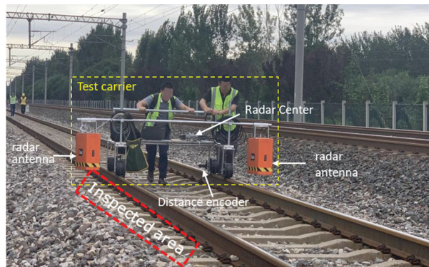
Figure 1. GPR equipment on a ballasted track using a 2 GHz antenna.
