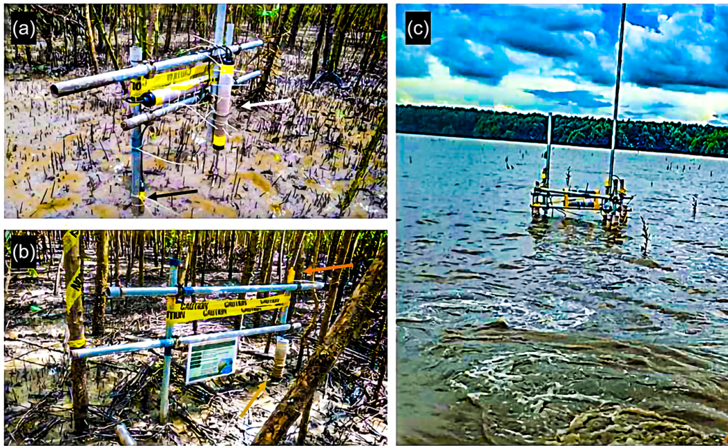
Figure 4. Simultaneous deployment of pressure transducers (gold arrows), acoustic Doppler velocimeters (white arrow), conductivity–temperature–depth loggers (orange arrow) and the optical backscatter sensors (black arrows) at the Chateau Margot transect (MB). (a) A view of station MB 3 in the sparser Avicennia -dominated forest approximately 110 m away from the concrete dyke. (b) A view of station MB 1 in the denser part of the Avicennia -dominated forest approximately 30 m from the concrete dyke. (c) A view of station MB 5 (located on the mudflat) used in the test deployment and field calibration of all of the instruments.
