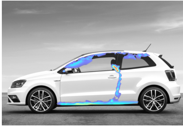
Figure 1.6: Applications of Acoustic Vector Sensor arrays - Sound visualization using two dimensional scan and paint approach.
