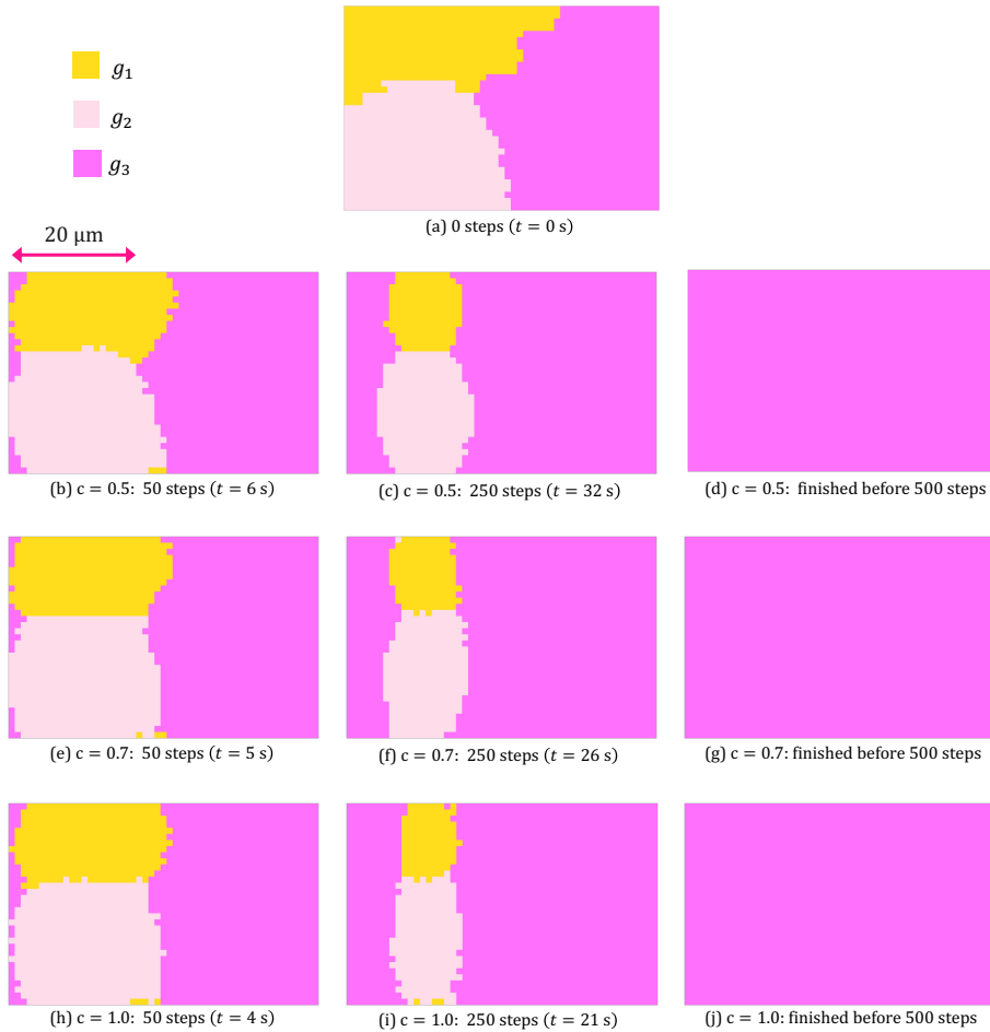
Figure 3.11: Tricrystal RVE at 1000 °C simulated in Sq(1,2): The maps show the evolution at (a) 0 time steps - 0 s (b) 50 time steps for c = 0.5 (c) 250 time steps for c = 0.5 (d) 500 time steps for c = 0.5 (e) 50 time steps for c = 0.7 (f) 250 time steps for c = 0.7 (g) 500 time steps for c = 0.7 (h) 50 time steps for c = 1.0 (i) 250 time steps for c = 1.0 and (j) 500 time steps for c = 1.0 .
