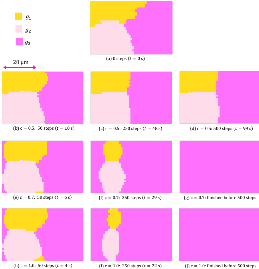
Figure 3.9: Tricrystal RVE at 1000 °C simulated in Sq(1,1): The maps show the evolution at (a) 0 time steps - 0 s (b) 50 time steps for c = 0.5 (c) 250 time steps for c = 0.5 (d) 500 time steps for c = 0.5 (e) 50 time steps for c = 0.7 (f) 250 time steps for c = 0.7 (g) 500 time steps for c = 0.7 (h) 50 time steps for c = 1.0 (i) 250 time steps for c = 1.0 and (j) 500 time steps for c = 1.0 .
