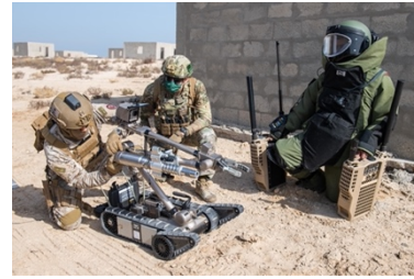
Figure 2: Packbot, a military search robot by Endeavor Robotics, has low autonomy in sensing and planning, but high autonomy in acting.
