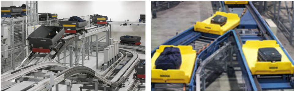
(a) Carts powered by linear induction motors. (b) Passive tubs on modular conveyor elements.
