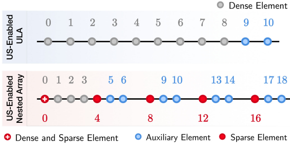
Fig. 2. Architectures for US-ASP using ULAs and nested arrays, for K = 2 . The spacing between sensors is normalized by d . The information provided by the auxiliary sensors (sensors lost when performing the spatial difference) is employed to access the unfolded samples. (Top) ULA array with L = 11 physical sensors and 9 effective elements. (Bottom) Nested Array with 4 effective elements in the first level and 4 effective elements in the second level. As it comes clear from the figure, the auxiliary elements are only required in the sparse subarray.
