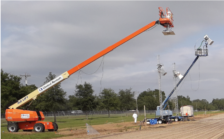
Figure 2.3: Scattermeters in Florida 2018 before sowing. The UF-LARS system is mounted to the blue crane (right).
