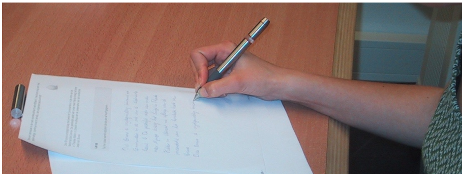
Figure 4b.5. One of the subjects writing with the biofeedback pen attempting not to light up the light signal at the top of the pen in order to minimise pinch force.
