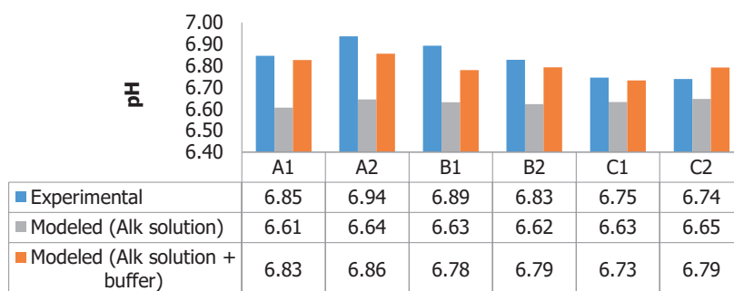
Figure A-4: Experimental and simulated results for equilibrium pH in physicochemical system at 3 bar \text{pCO}_2 using a different types of inoculum: A) Sludge from UASB treating waste activated sludge from a domestic wastewater treatment plant B) sludge from a UASB treating effluent from a sugar beet factory and C) Sludge from an AnMBR treating wastewater from the food and feed industry
