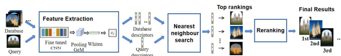
Fig. 1. Proposed pipeline. First, features are extracted from the query image. Similarly, such features are also extracted from all images in the database. These features are extracted only once, and are then stored for processing the image-based queries. The feature extractor comprises a CNN, followed by an aggregation layer, a whitening layer and an L2 normalization layer, which can be trained end-to-end with various loss functions. The extracted features are then forwarded to an approximate nearest-neighbour search module to produce the initial ranking results, which are next refined by a re-ranking module, generating the final results.
