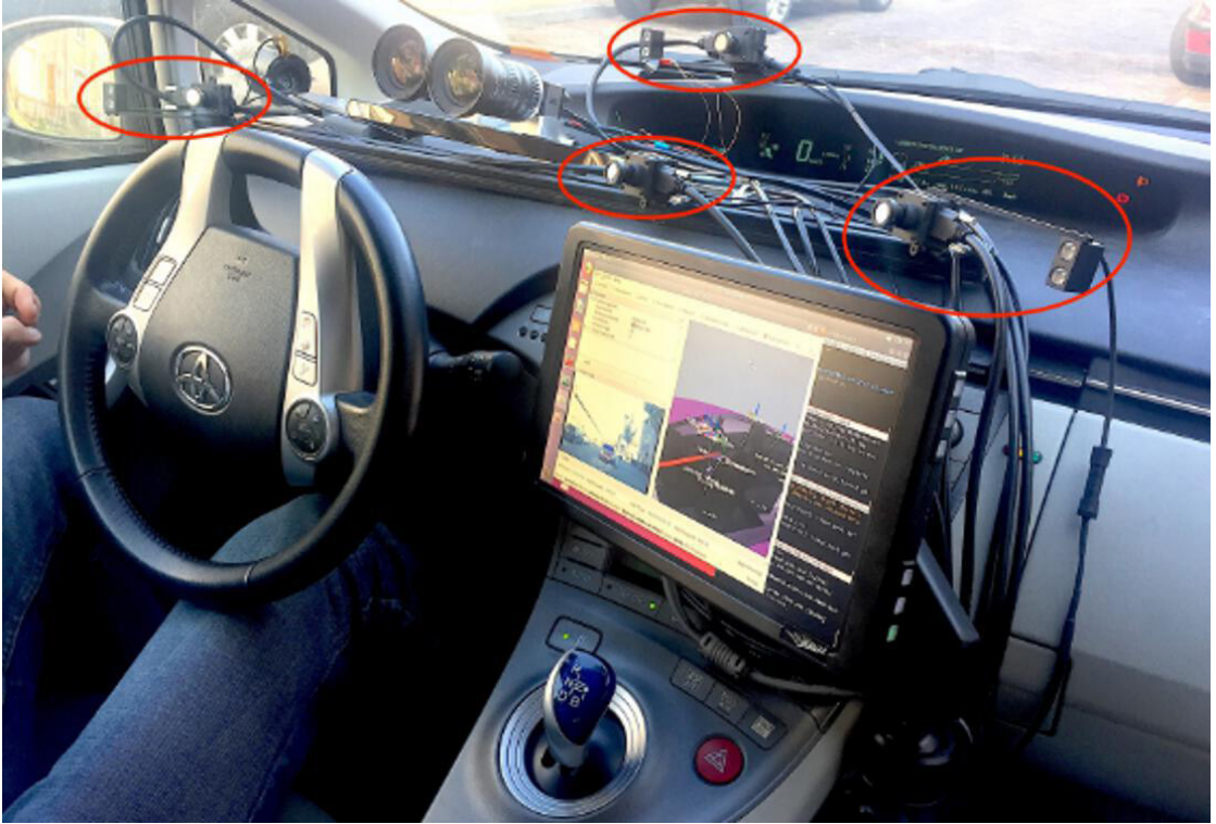
Figure 1. Interior of the vehicle showing the four eye-tracker cameras encircled, and the built-in display used for the post-drive recognition task.
