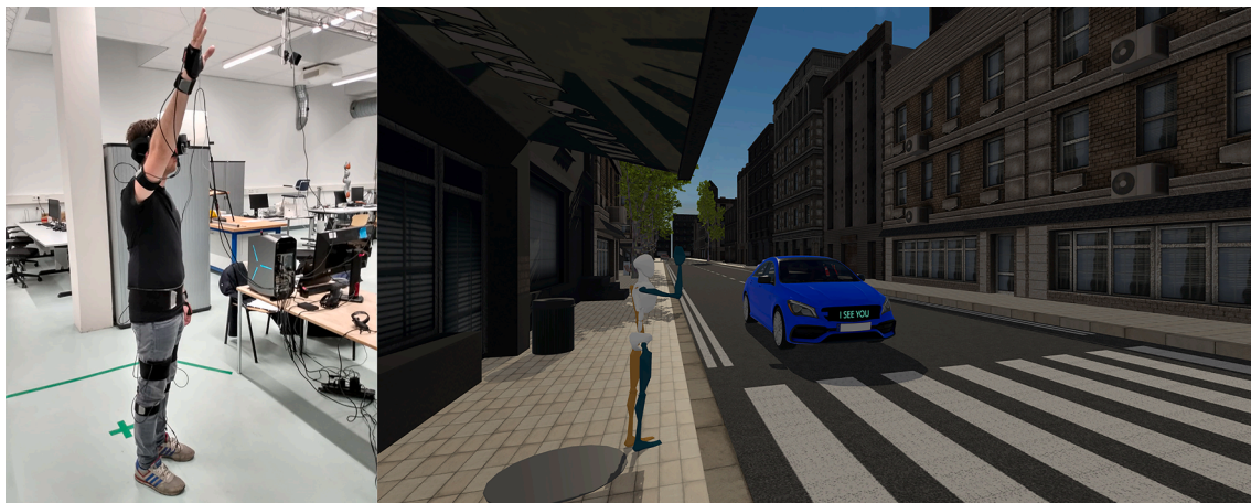
Fig. 3. Hand gesture towards the AV (left) as an indication that the participant wanted to cross, and the virtual-reality environment with eHMI on AV displaying I SEE YOU and an avatar visualizing the participants' body (right) (Epke et al., 2021).
