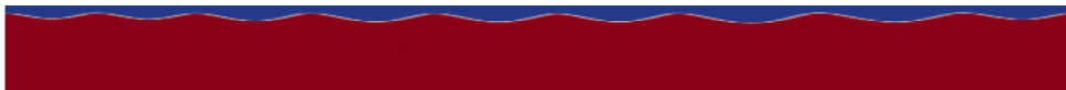
Figure 6. Example result showing the preferred wave length when the streamwise length of the considered pipe section is increased.
