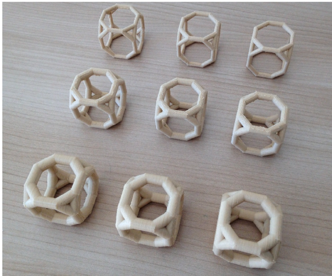
Fig. 9. The additively manufactured unit cells having equal strut length but three different thicknesses.
