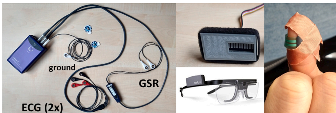
Fig. 1. Overview of physiological sensors, eye tracker, pressure sensor for continuous subjective rating and LED bar for visual feedback of pressure sensor.
