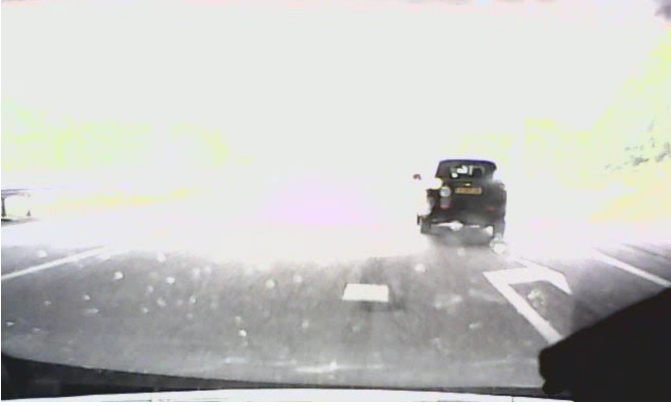
Figure 4.4: The ego vehicle passes a flyover during daytime while performing a lane change. This causes glare such that the distance to the lane lines are temporarily unavailable.
