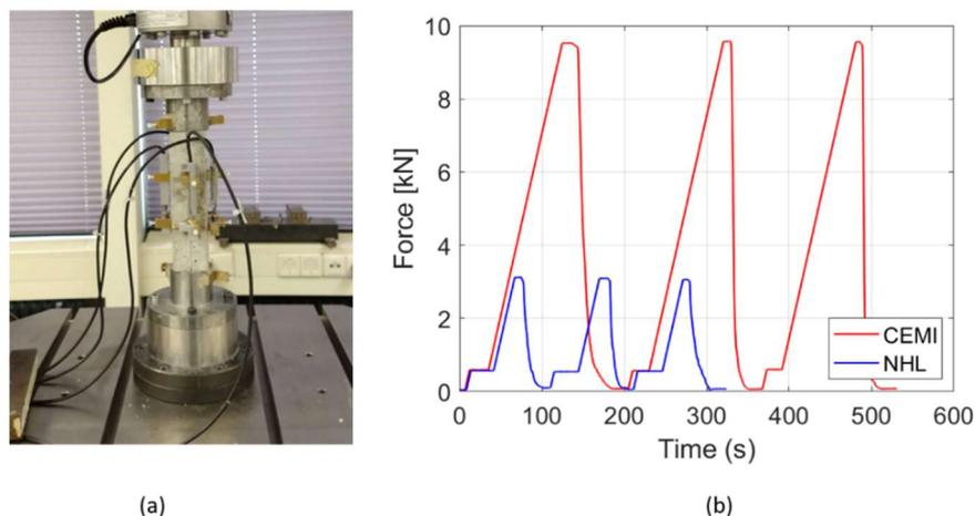
**Figure 1.** (a) Experimental setup for measuring Young's modulus. Displacement measured using LVDT (b) Applied loading-unloading cycles for E-modulus measurements.
